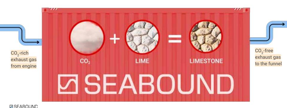
Seabound Containers connect to a ship's exhaust with minimal retrofits. At port, saturated containers are swapped for fresh ones — just like regular cargo.
