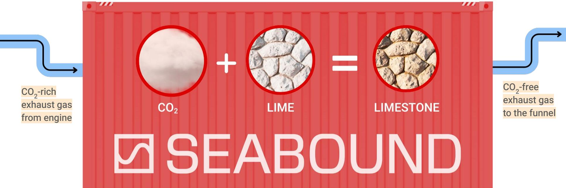
**Seabound Containers connect to a ship's exhaust with minimal retrofits.** At port, saturated containers are swapped for fresh ones — just like regular cargo.
